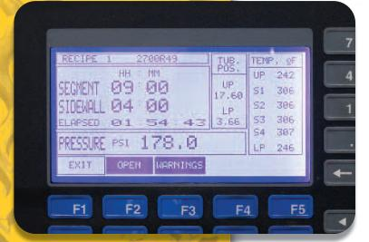
Just as in new tire production, our tires are cured in a segmented mold. PLC logistics control time, pressure and separate temperature zones for the bead/sidewall area and tread area.
