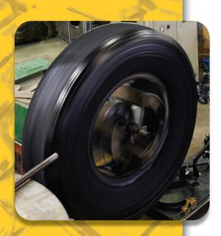
Radial tire retreading requires that the tire be built to precise dimensions. In order to achieve this, we utilize computer-controlled building machines which wind a continuous ribbon of rubber around the buffed tire. As in the buffing process, the operator chooses from a variety of programs for each tire size and design.
