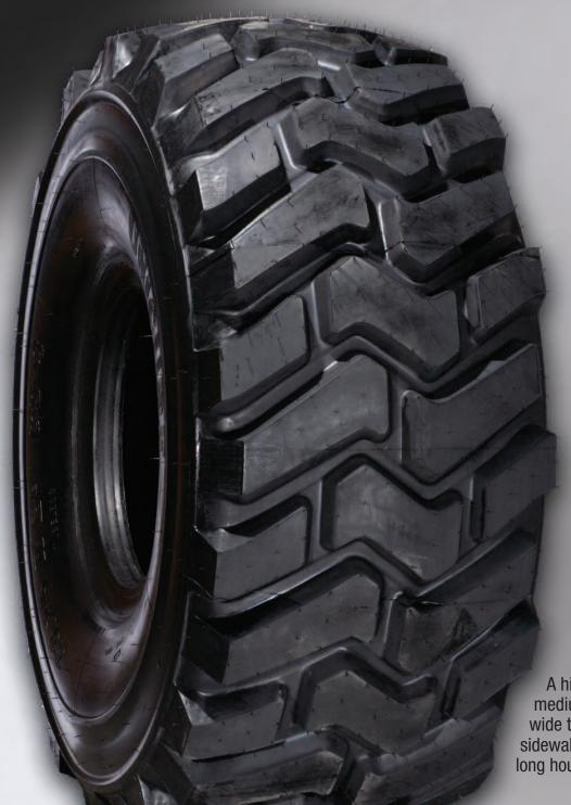
A high traction design for medium size scrapers. The wide tread provides extra sidewall protection and gives long hours of service. Unicure 62
