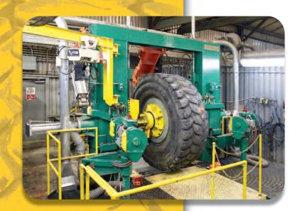
With our system, all tires are buffed inflated on a computer-controlled buffer. CNC technology allows us to buff each tire to an exact diameter and profile to ensure uniformity.
